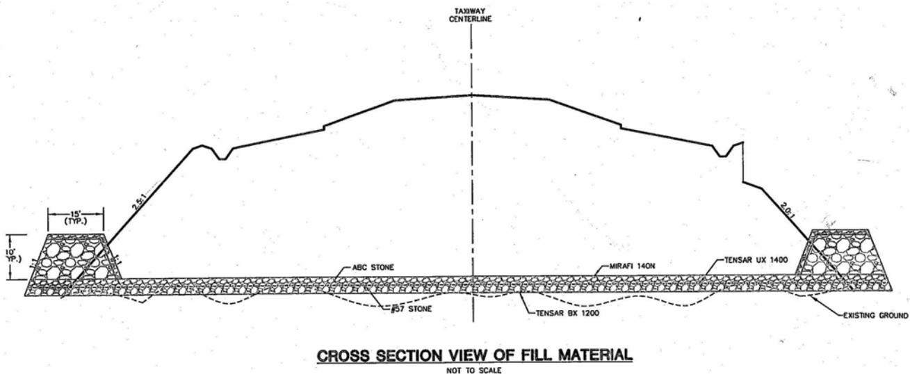
Figure 2. Cross Section View of Fill Material
